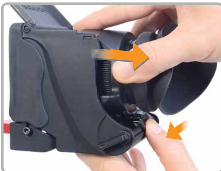
Press the locking lever and remove the loupe.
