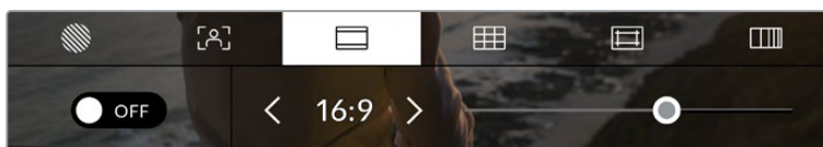
Tap the 'frame guides' icon while accessing 'LCD monitor options' to access your URSA Mini's frame guide settings
