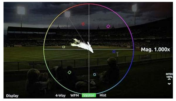
Color saturation is determined by the distance from the center of scope - the more saturated (vivid) a color, the further its trace reach is from the center. A grayscale image should appear as a dot in the center of the scope.
