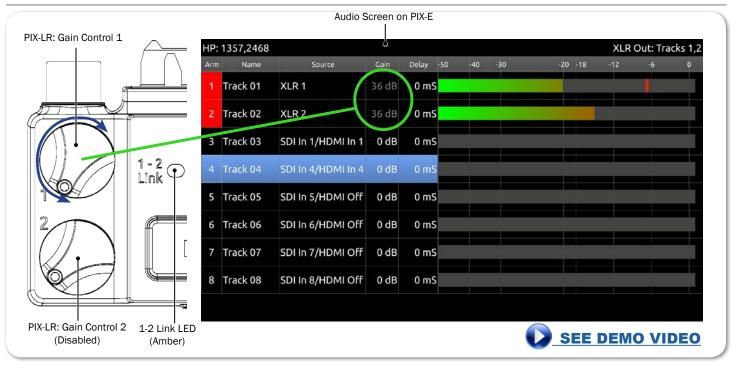
As shown in the previous illustration, when linking is set to 1-2 Linked without Pan, gain control 1 adjusts the overall gain level of both XLR inputs, while gain control 2 is disabled.
