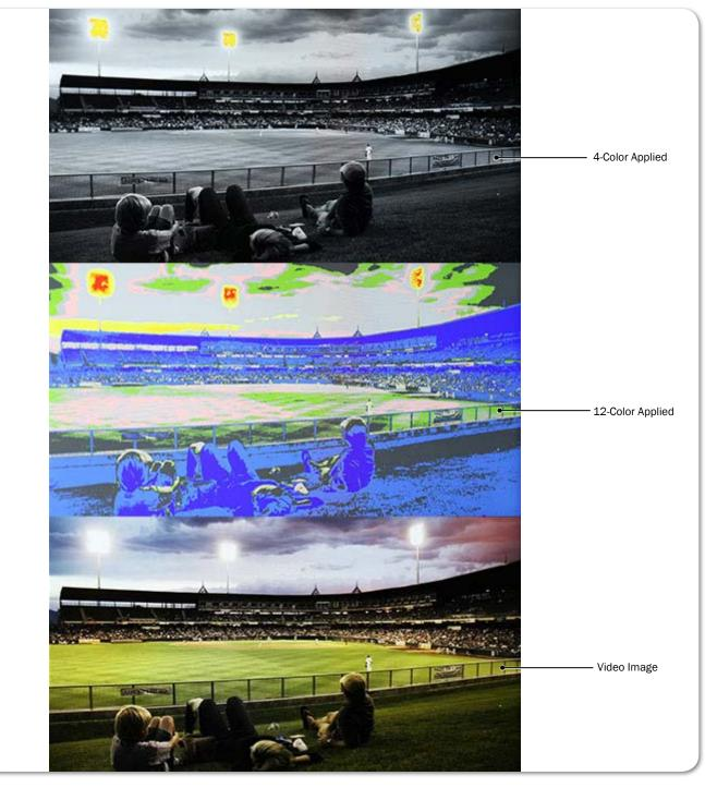
The 4-color mode is ideal for quickly identifying over- and under-exposed regions. Under-exposed regions are highlighted blue and over-exposed regions as yellow or red. All exposure levels in between are displayed as grayscale.
