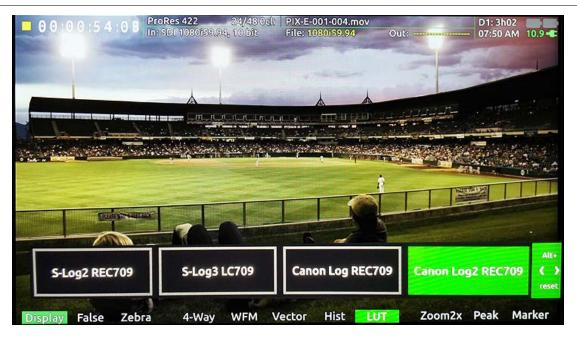
The LUT menu appears superimposed over the image, along the bottom of the screen, with four LUT options. The currently applied LUT appears highlighted in green.
