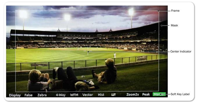
A frame marker is a thinly lined rectangle used to "frame" the shot. The frame may be customized to match the aspect ratio of the video, such as 16:9 for high-definition television. The area within the rectangular frame is safely "inside" the shot; the area outside the rectangle is the mask, which is considered "outside" the shot. There are two frame markers available on the monitor, which may be configured separately.
