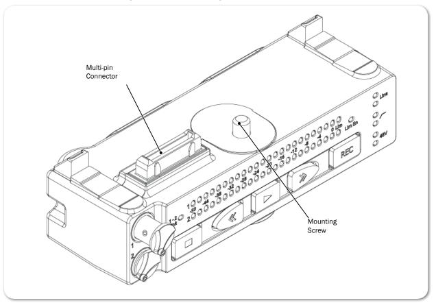
The PIX-LR attaches to the bottom panel of PIX-E monitors. Sound Devices, LLC recommends, as a best practice, the monitor's power be turned off and unplugged before affixing the accessory. Further instructions for attaching the PIX-LR to your monitor is provided in the <u>PIX-LR Quick Start Guide</u>, which is shipped with the accessory. It is also available as a free PDF download from the Video Devices website.
