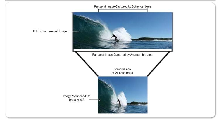
The PIX-E monitors have the ability to "desqueeze" an image to the LCD and SDI/HDMI outputs during both monitoring input and playback. The process stretches out the horizontally squeezed images that result from cameras using anamorphic lens so that objects in the images, when displayed on the LCD or via outputs, do not appear elongated and thinned.
