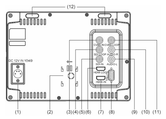
(1) DC 12V IN: Connect with DC12V 4-pin XLR power adapter. (Pin 1: Negative, Pin 4: Positive)
