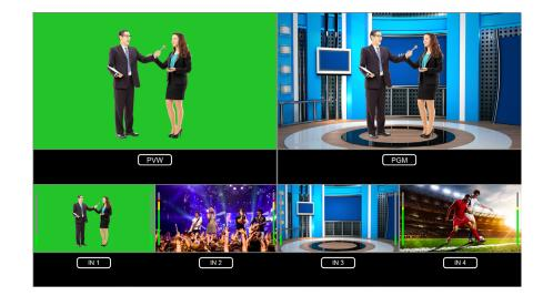
You can monitor all sources at the same time on a screen through ez-Pro VS4. The multiview allows easy monitoring of all video inputs, audio levels, the preview (PVW) and the program (PGM) screen without confusion. Picture-in-Picture (PIP) can also be repositioned and resized on the multiview screen.
