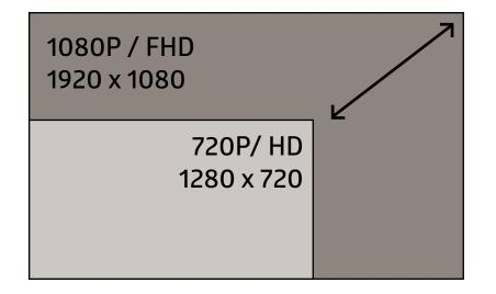
Each video input has a built-in scaler that can be set up to 1080p. The incoming video source resolution will be automatically displayed on the LED screen. The output program (PGM) can be up/down scaled to any HD resolution up to 1080p.
