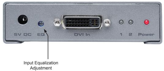
The external equalization knob can be used to balance out signal noise resulting from long cables for better picture quality. By turning the equalization knob counter-clockwise you will eliminate any noise and/or degradation in the signal. You should be able to find a "sweet spot" somewhere in the middle.
