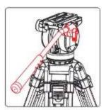
Pan Arm can be removed and positioned on opposite side of head: An optional Pan Arm can also be mounted to provide dual control.
