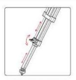
Flip Leg Look Levers down and side Leg sections to adjust height. Flip Levers up to look.
