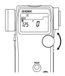
When the light from the flash is received, the measured value (f stop) is displayed. Each time this is repeated, the accumulated value for the aperture and the number of cumulative flashes is displayed.
