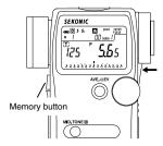
1) After taking a measurement by pressing the Measuring button pressing either the Memory button putton putton or AVE./ EV button stores the measured value as zero in the middle of the EV scale representing the MID.TONE value. Pressing MID.TONE button will display a blinking " A " on the scale. Pressing AVE./ EV button will display a blinking " To not he scale.
