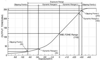
It is necessary to test the cameras sensitivity, measure the actual dynamic range and know the clipping points of your digital camera and/or type of film and processing used before programming the L-758DR (L-758D/L-758CINE) meter for Exposure Profiling. Film exposures should be evaluated by scanning the film first and then evaluating the images in a photo application software. The use of a transmission/reflective densitometer can also be used if film scanning is not possible or desired.
