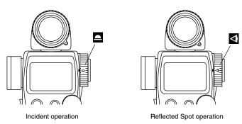
When incident operation is selected, the mark will blink for ten seconds and when Reflected Spot operation is selected the mark will blink for ten seconds on the LCD.
