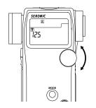
Press the Measuring button to trigger the flash.
