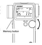
4. Turn the main lighting off. Now, point the Lumisphere toward the secondary light source. While pressing and holding the Measuring button , the indicated difference between the main and secondary light source is displayed in EV. At the same time, the standard value and a new measured value are displayed on the analog scale.
