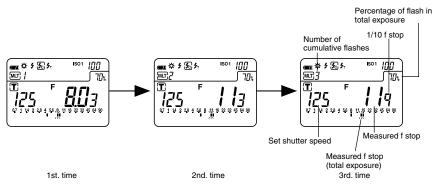
To clear the cumulative value, press M. CLEAR button @ or switch to another mode by turning the Jog wheel while pressing the Mode button.
