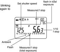
5. When the light from the flash is received, the measured value (f stop) is displayed. Even after measurement, the mode mark 3 continues to blink and the meter is in ready state and a new measurement can be made. (Auto-reset function)
