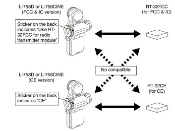
Be sure to purchase either RT-32FCC or RT-32CE module according to your light meter's destination. Old RT-32 module cannot be used with L-758D or L-758CINE.
