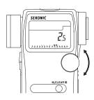
11) Setting Clipping point (+) Rotate the Jog wheel while pressing ISO2 button . Clipping point can be set from 0 to +7EV in 1/10 step increments.
