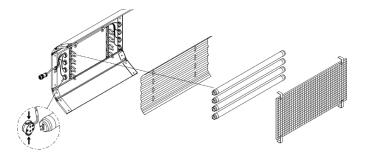
The 4Bank, Double and Single fixtures are comprised of a removable Louver, Reflector and Lamp Harness. The Louver and Reflector are held in place with Velcro fasteners. The Lamp Harness is secured by means of a ¼ turn fastener and two clips.
