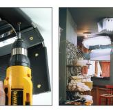
The grommet holes along the edge of the fixture are designed to allow the fixture to be screwed onto set walls.
