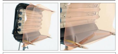
Restricting the airflow around the lamps can cause the lamps to operate hotter. This increased heat will raise the lamp's color temperature and green spike. Therefore, it is recommended to clip gels to the doors of the fixture.
