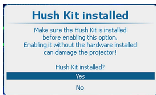
Image 11-7 Confirm Hush Kit physical installation.
