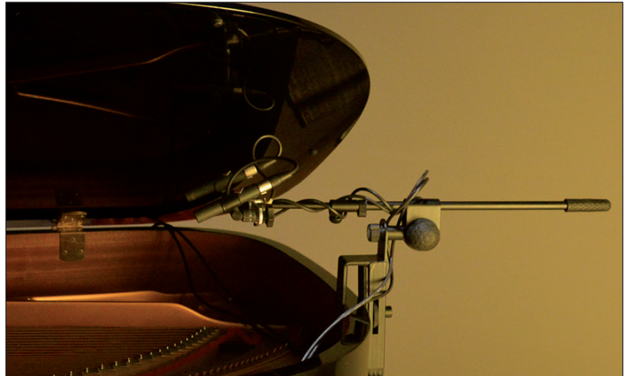
A/156 mic boom arm, anchored to the piano body, with MP/900 dual mic holder. Microphones are positioned within the piano body to achieve a more direct and higher-definition sound pickup.
