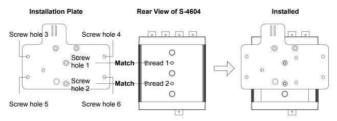
Match the screw holes 1&2 with the threads 1&2 of S-4604, and fix the installation plate to the S-4604 by the supplied screws. The screw holes 3, 4, 5, 6 are used to install S-4604 to wall or racks.
