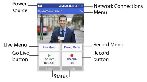
The Preview screen is the hub of the EnGo transmitter. The touch screen shows the live camera feed, as well information about the power level, network connections, stream health and any errors. You can also use the screen to broadcast live or record clips quickly. On the Preview screen, you can start a broadcast or record Store & Forward clips with a quick tap of the Go Live or Record buttons.
