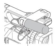
Put the cable in the outer cable holder.
