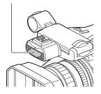
1 Set the CH-1 (INT MIC/EXT/MI SHOE) switch D and CH-2 (INT MIC/EXT/MI SHOE) switch H to "INT MIC."
