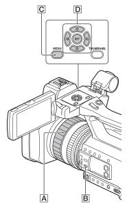
1 During recording or standby, press the FOCUS AUTO/MAN button B to set the focus to manual.
