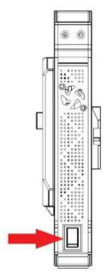
4. Press "CH" button to select the corresponding working channel of receiver and then press "OK" button for confirmation. The LED digits display will display one of the characters from 1 - 9, A and b when the video signal of device is normal; the monitor will display the image from camera simultaneously.
