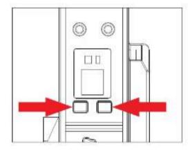
5. The transmitter supports manually switching the SDI audio input mode by long pressing "OK" button. (Notice: This function is only valid for SDI audio input and won't affect the HDMI audio input.) The default value of SDI audio input mode is 0 and the decimal point will be set to be non-bright under this mode; long press "OK" key button for more than 3 seconds, and then the LED digits display will display SDI audio input mode as 1 while the decimal point will be bright.
