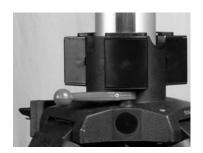
As some pressure is already applied at the factory, the centre column may now move upwards. You can check the pressure with the pressure gauge at the column.
