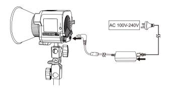
\* Please press the spring-loaded lock button on the power cord to remove the power cord. Do not pull it out forcibly.
