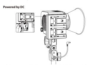
\*The batteries are not included. Please press the spring-loaded lock button on the battery plate to remove the power cord. Do not pull it out forcibly.
