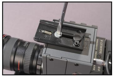
After lining up the Dovetail Quick Release Plate to the thread inserts on the bottom of the camera, use a ½-11 or 3/8-11 screw to attach the plate to the camera. (See *figure 23*)
