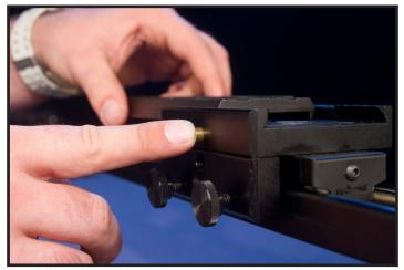
Gently push in the brass button in, then, carefully slide out the Dovetail Quick Release Plate.
