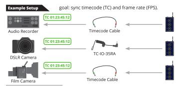
NOTE: Required cable depends on connected device. E.g. TC-IO for ARRI, LTC-Out/Epic for RED, LTC-Out for CBMC, Canon, Panasonic, Sonv. Please check our website.
