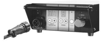
Connect the same way the other end of the extension cable in the input receptacle coming out from the lamp head.
