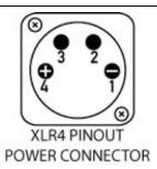
When powering the 4LIGHT through the XLR4 connector located at the back of the VDC Control Unit check the proper polarity as shown in the picture at the Control Unit bottom.
